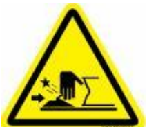
WHEN CLAMPING THE RIM, DO NOT PLACE HAND OR OTHER PARTS OF THE BODY IN BETWEEN THE CLAMP & THE RIM.
