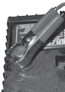
FIGURE 11 Red Positive (+) to Battery
