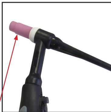
(9) Assemble front end parts of the TIG torch, fitting a sharpened tungsten suitable for DC welding.
