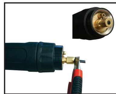
(9) Cut the liner flush with the end of liner retaining nut using a sharp box cutter knife.
