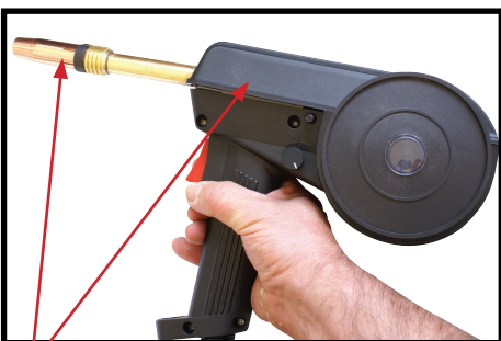
(15) Fit the gas nozzle and close the wire feed spool cover
